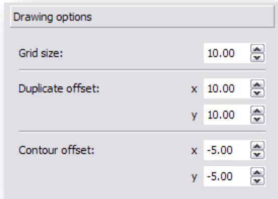
**Grid size** – This value sets the distance between the gridlines in both vertical and horizontal direction.
